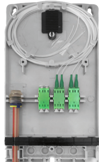
SDU-Wallbox-SP Exemplary full occupancy for supported expansion with LC/APC adapters and pigtails plus input with cable protection tube
